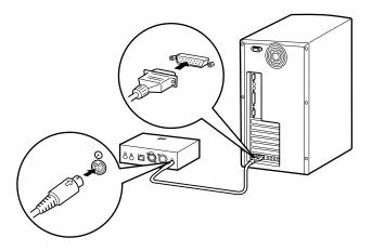
As shown in the illustration on the left, begin by connecting one end of the PC connector cable to the joystick/MIDI port of your computer's Sound Blaster 16 card and the other end to the "PC" connection on the IF6P.
